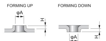
Forming process for making tubes of threading for screw. Threading for screws and increased bearing area for tubes.
