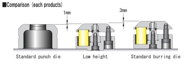
Note: Maximum thickness of material is 1mm. Stainless steel does not fit to this apprication.
