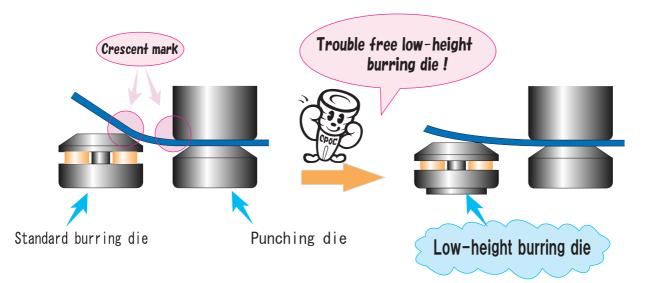
Low-height burring die is just 1mm higher than standard punching tool. Therefore it is possible to punch next of burring tool also avoid scratch from material movement and turret rotation.
