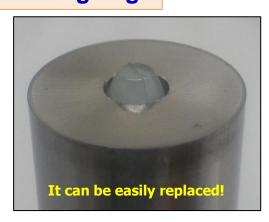
Slug Ejector is a consumable item. When regrinding, replace it with a new one!
