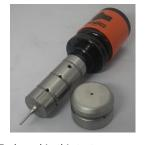
Tool used in this test PROTECH3 1-1/4'' Standard round set  $\phi 3.3 \ C = 0.3$
