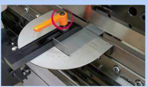
\*If the clamp lever interferes with the punch or brake, it can be changed to any position by pulling up and turning the lever.
