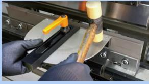
2. Use a plastic hammer to adjust the position of the front table of the main unit and the top surface of the die so that they are aligned.
