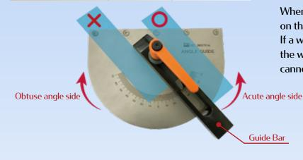
When machining angle bending, place the workpiece on the acute angle side of the front table. If a workpiece is placed on the obtuse angle side, the workpiece will interfere with the guide bar and cannot be processed.
