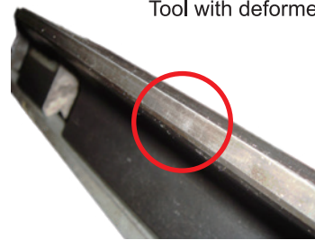
Tool with deformed bending edge
