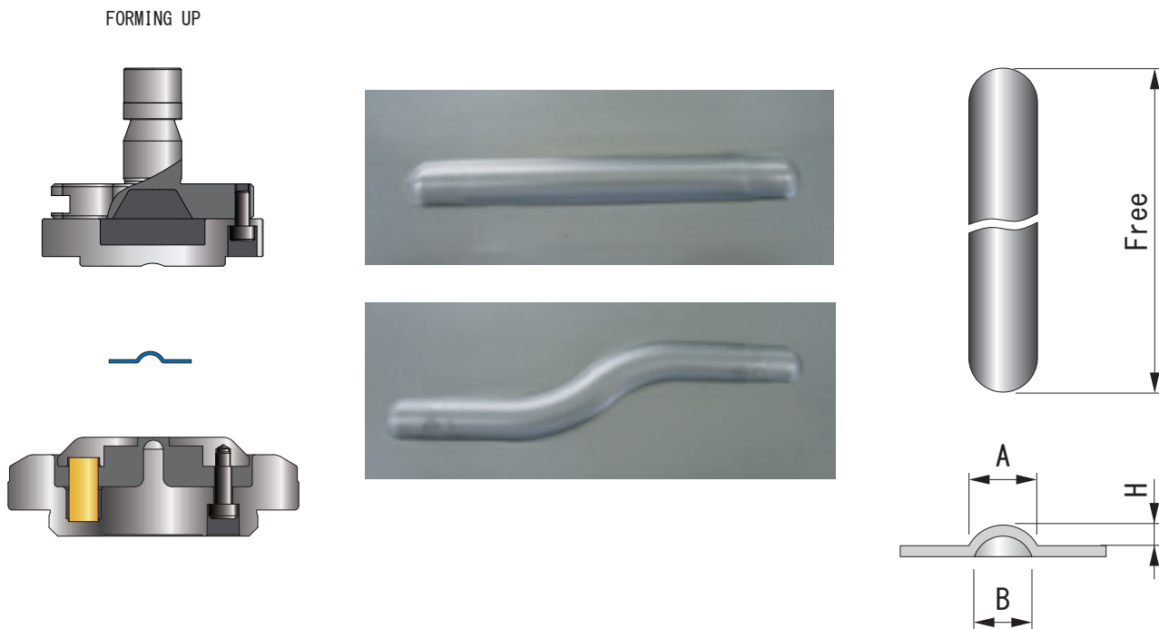
Forming process of embossing that can hit continuously along the sheet. Used for strengthening, nonslip or decoration.
