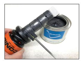
In particular, apply carefully to the outer circumference near the root of the cutting edge and near the retainer collar.
