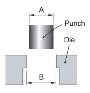
When specifying the clearance of the die, please indicate whether it is a clearance on both side or one side. Or you can also specify dimensions with clearance.
