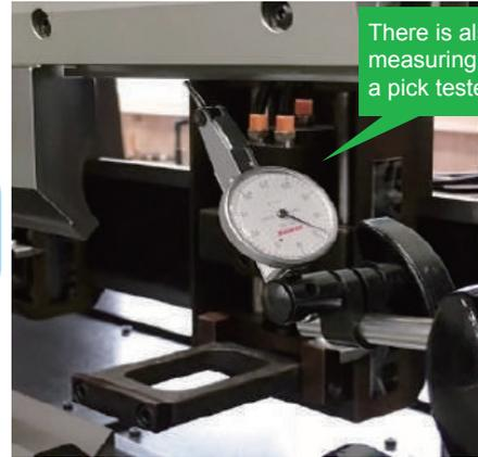
There is also a method of measuring parallelism using a pick tester.
