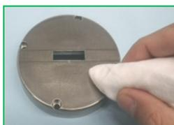
① Oil and dirt on the surface on which a sticker will be put should be removed completely by thinner or the like.
