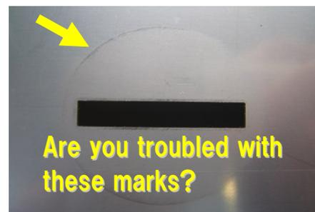
**Mark-less sticker reduces marks on the surface of workpieces made by punch press tools and improves the quality of sheet metal processing. It is a special sticker and realized "easy sticking" and "Low cost". It is replaceable!!**
