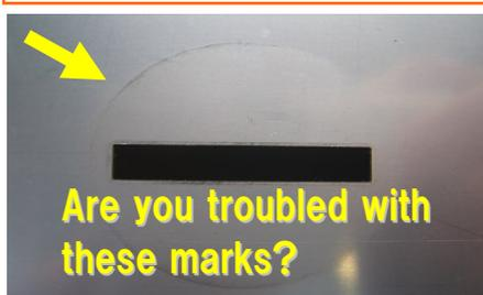
Mark-less sticker reduces marks on the surface of workpieces made by punch press tools and improves the quality of sheet metal processing. It is a special sticker and realized "easy sticking" and "Low cost". It is replaceable!!
