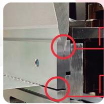
Process 1: Sharp angle bending
