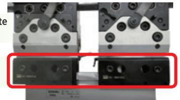
Mounted under the Amada intermediate plate, the higher punching height allows for deeper bending
