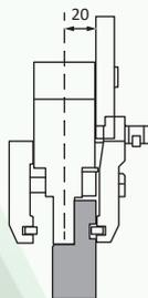
Easy clamping by simply operating the handle.
