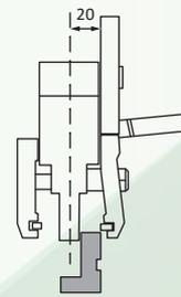
All types of tooling can be released. It is convenient for changing the short toolings in the center.
