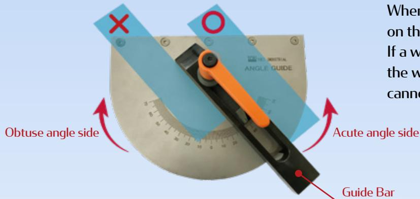
When machining angle bending, place the workpiece on the acute angle side of the front table. If a workpiece is placed on the obtuse angle side, the workpiece will interfere with the guide bar and cannot be processed.
