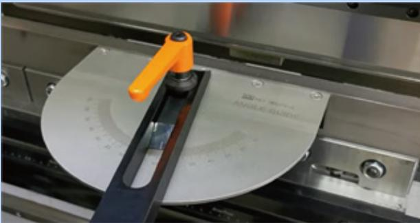
3. Align the scale line on the guide bar with the desired angle and start machining by placing the workpiece against the guide bar.
