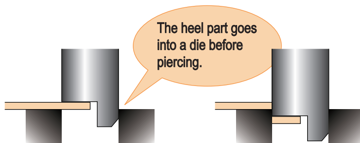
Fig.3 Prevention of punch misalignment with heeled tool
