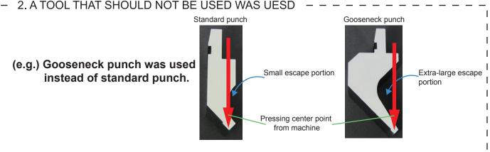
Bending with a standard punch, compared to a gooseneck punch, has less deflection and better accuracy as the "C shape" of the tool relief is smaller.
