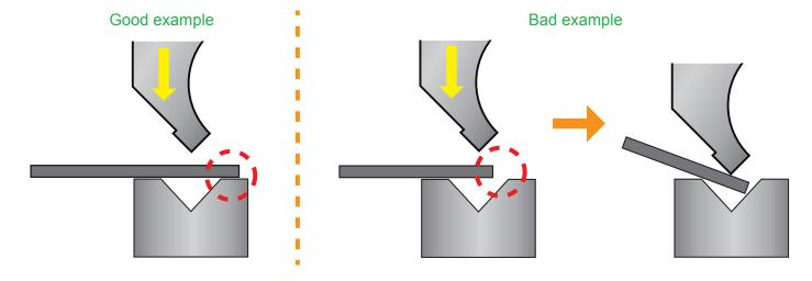
**Method 1:** Calculated with Minimum flange length (b) = 0.7V (V = V-width of die)
