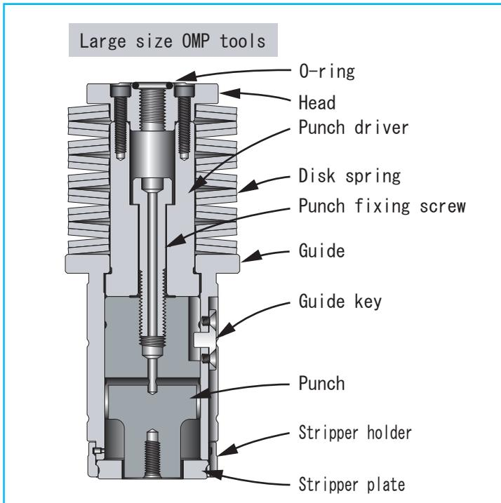
OMP punch is designed for anti-seize and long life the tools by using oil mist put into punch slide area and punching edges.
