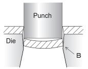
② The slug is compressed in the process of punching at [B] part.
