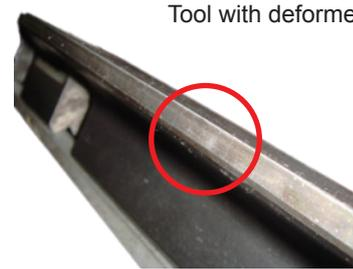
Tool with deformed bending edge
