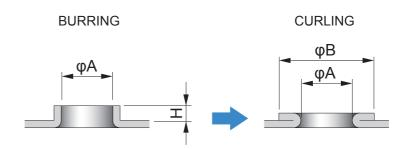
Forming process to bend the material after forming of burring. Used to guide or protect the code and pipe.
