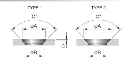
Forming process of making a chamfer to material. Used for sink a countersunk screw head, make chamfer to a corner
