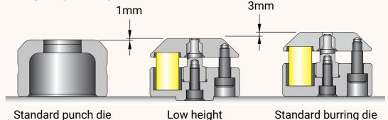
Note: Maximum thickness of material is 1mm. Stainless steel does not fit to this apprication.
