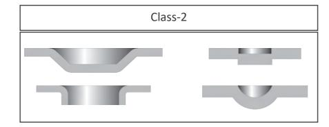
Typically, the height of upward burring dies is significantly higher than that of standard punching tool dies. As a result, the difference in die height can cause crescent-shaped marks on the material.
