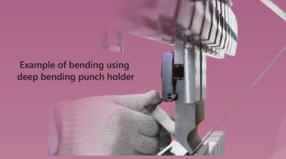
When performing deep "U-shape bending" or "hat-type bending," the new system eliminates the problem of workpiece interference with the intermediate plate or upper table due to insufficient stroke of the conventional punch height.
