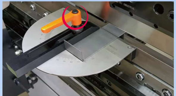
*If the clamp lever interferes with the punch or brake, it can be changed to any position by pulling up and turning the lever.
