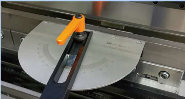
3. Align the scale line on the guide bar with the desired angle and start machining by placing the workpiece against the guide bar.
