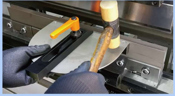
2. Use a plastic hammer to adjust the position of the front table of the main unit and the top surface of the die so that they are aligned.
