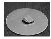
The guide part is formed on the edge of the Z-bending.
