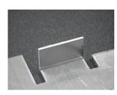
L forming of the end of a workpiece.
