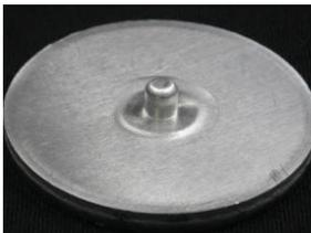
This is the example when 80% of the material thickness is rose. Generally, in consideration of the hardness, the material is rose within 60% of its thickness.
