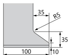
耐圧 1000kN/m (100ton/m)
