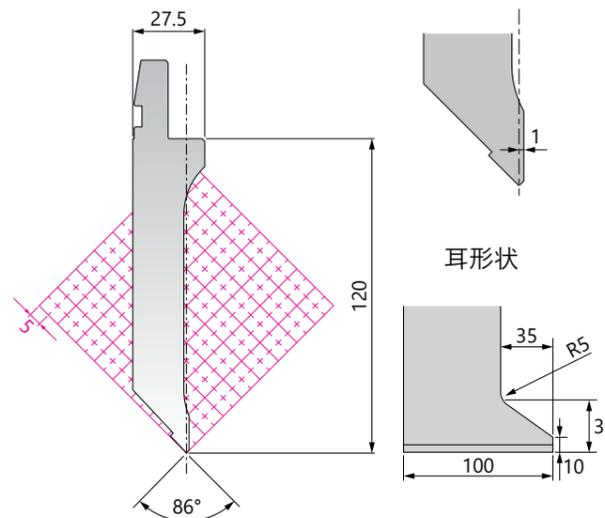
耐圧 800kN/m (80ton/m)
