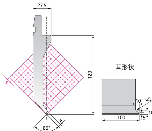
耐圧 200kN/m (20ton/m)
