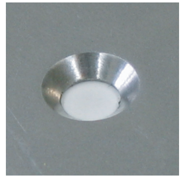
Fig.1 Chamfering formed by press
