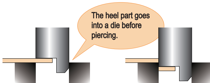
Fig.3 Prevention of punch misalignment with heeled tool
