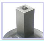
The state of the cutting edge after 1.8 million hits at Company B shown below.
