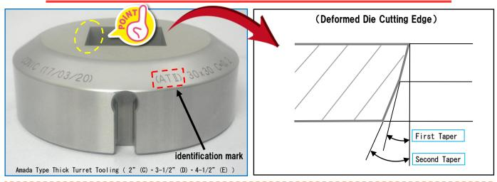
This die cutting edge is suitable for a punching machine with slug vacuum function, which discharges punched slug strongly to scrap boxes. This die maximizes slug suction function and prevents slug pulling for large station.
